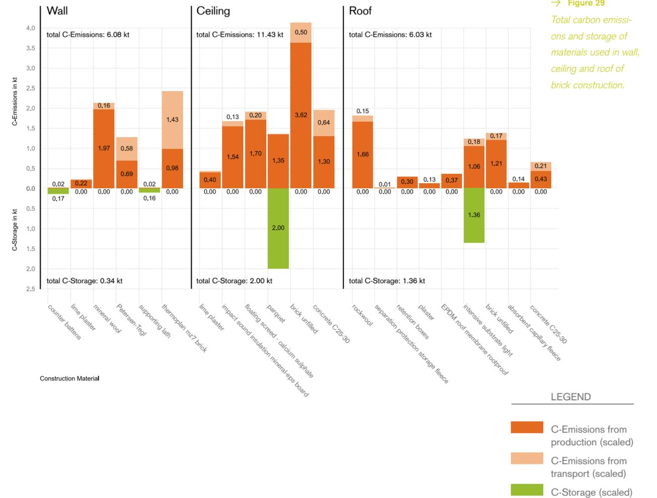
→ **Figure 29** Total carbon emissions and storage of materials used in wall, ceiling and roof of brick construction.
